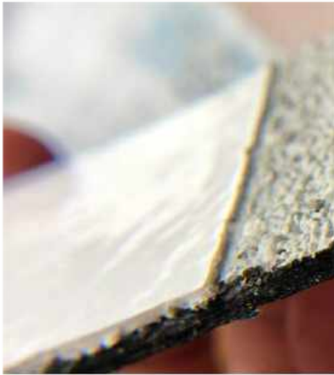
DISADVANTAGE: ROOF COATING ONLY PROVIDES WATER BARRIER CONTAINING NO REINFORCING FIBER.
